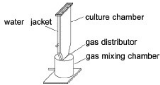
Figure 2.6: Experimental thin-layer flat-plate photobioreactor (Xu et al., 2011).
